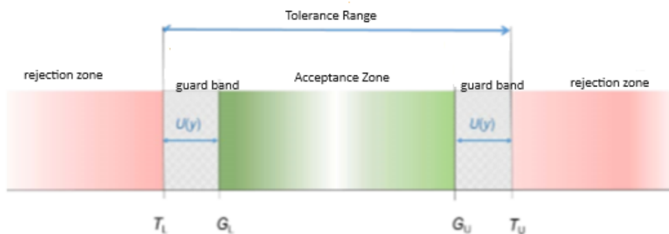
Figure 3- Acceptance and Rejection Zone Based on Lower and Upper Limits (False Acceptance)
